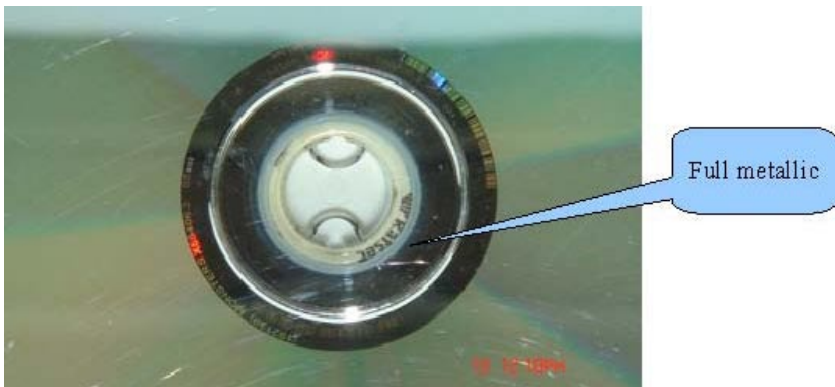
Illustration 6: RFID detection is almost zero when the DVD centre is fully metallic
