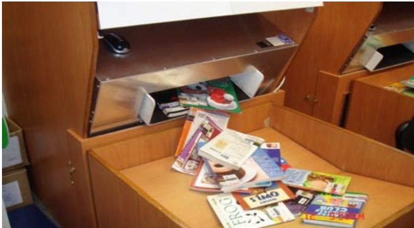
Illustration 4: NLB first generation RFID library system book drop (jammed)
