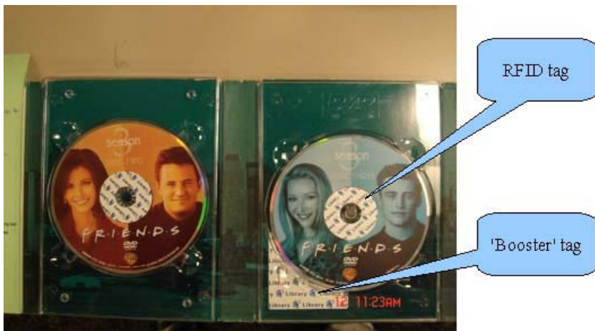
Illustration 5: DVD with booster tag and RFID tag
